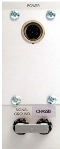
Figure 4: Rear panel connectors of the EPMS-E-07
