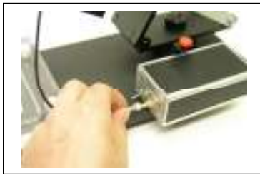
Connecting the recording electrode
