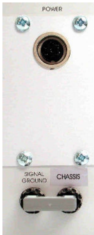
Figure 4: Rear panel connectors of the EPMS-E-07
