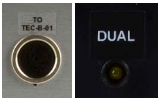
Figure 3: Rear panel connector of the BA-03X for connection with TEC-B-01 (left). A DUAL LED on the front panel of the BA-03X indicates two electrode operation (right).
