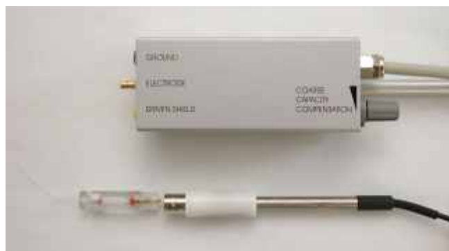
SEC standard headstage with electrode holder and adapter
