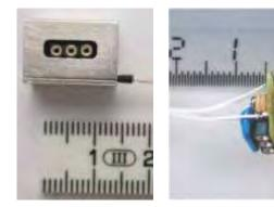
Mini headstages for putting directly on the animal's head, e.g. in freely moving rats
