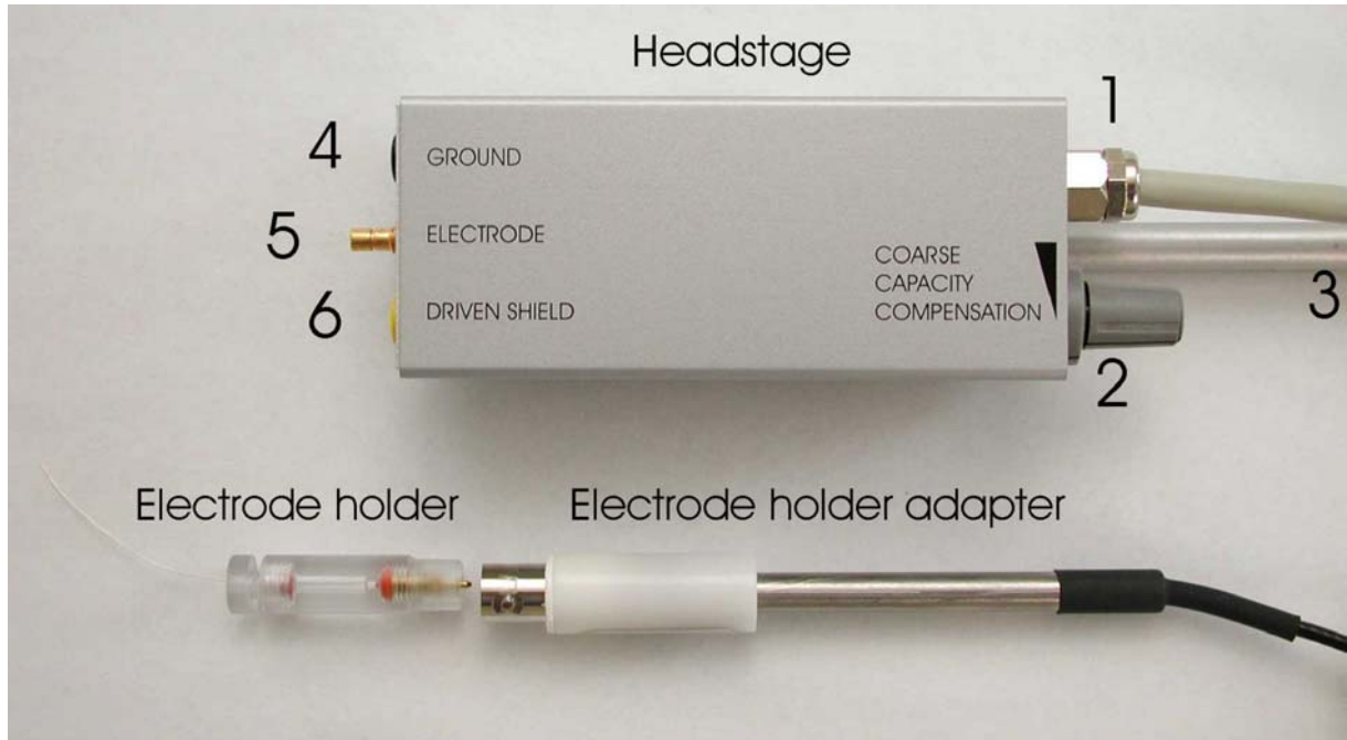
Figure 11: standard headstage, electrode holder (optional) and electrode holder adapter (optional) of the SEC-03M
