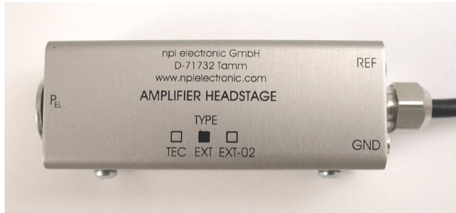
Figure 4: one headstage of the EXT-T2
