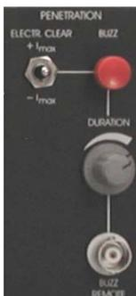
The PENETRATION unit consists of (13) ELECTR. CLEAR switch, (14) BUZZ push button, (15) DURATION potentiometer and (19) BUZZ REMOTE connector.
