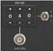
The gated stimulus unit consists of **(26)** + / 0 / - switch (STEP SIZE switch), **(27)** GATE (TTL) connector and **(28)** STEP SIZE digital potentiometer.
