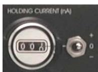
The HOLDING CURRENT unit consists of (10) HOLDING CURRENT (nA) potentiometer and (11) + / 0 / - switch (holding current switch).
