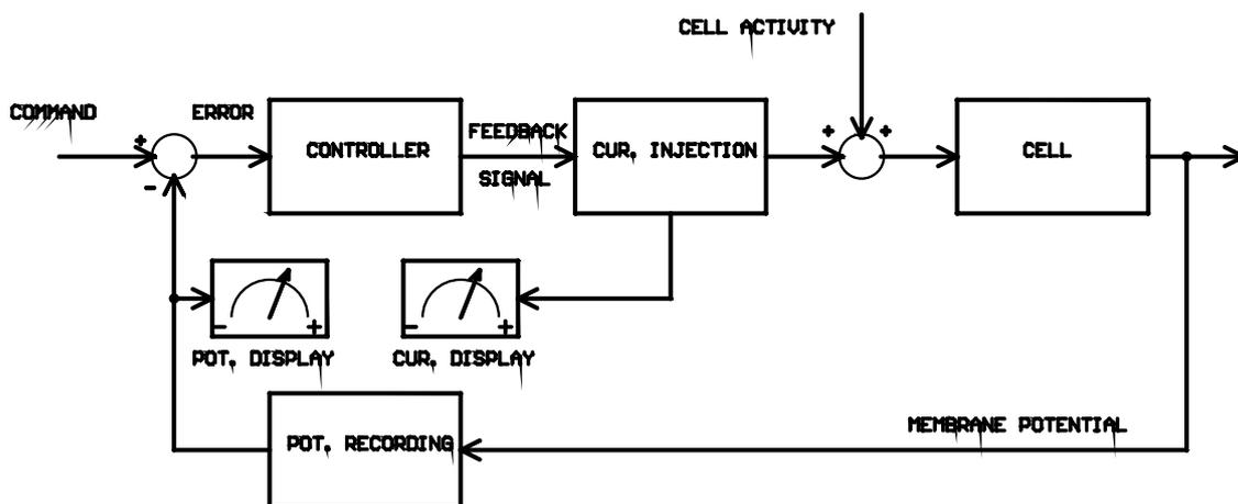
Fig.2B BLOCK DIAGRAM OF VC MODE
